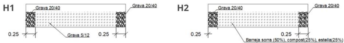
Figure 3. Horizontal subsurface flow treatment wetland description.
