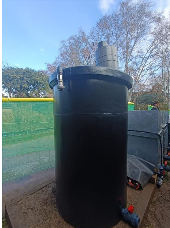
Reservoir tank with agitator
