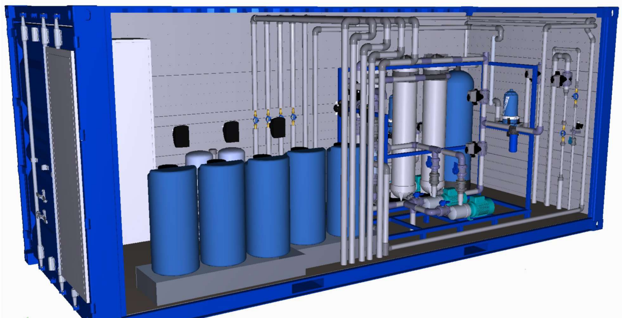
Figure 7 - Container water treatment plant
